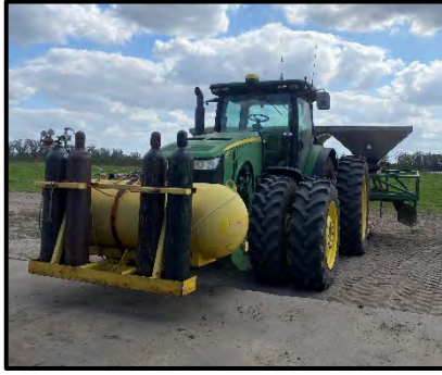
Closed system for application of TELONE™ using “pig” tank and cylinders to hold fumigant, and nitrogen pressure system.
