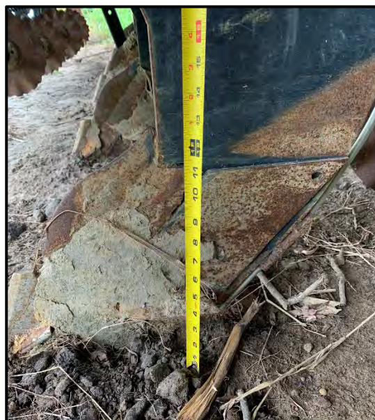
The reach nematodes where they live, inject TELONE™ at least 12"-20" below the final soil surface (measured from the bottom of the outlet tube). Deeper placement is recommended to control deeply distributed pests.
