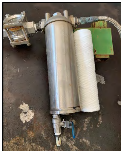
Regularly replace in-line filters.
