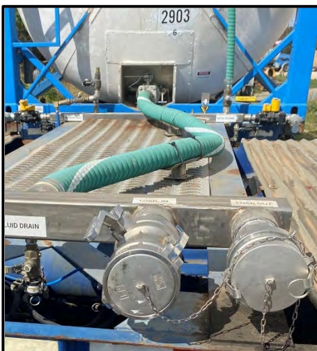
When not in use, keep dustcaps on all male and female dry-disconnect couplings to protect seals.
